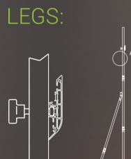
Designed for positioning the screen on the floor, they are made of matt, anti-reflex, high-resistance aluminium. The extension is obtained by rotating the upper profile which features some holes to anchor the screen at different levels. The floor anchoring is possible thanks to the horizontal segments which can be lowered separately.
